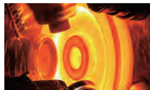
智能辗钢车轮生产线 —车轮轧制 Wrought steel wheel intelligent production line—wheel rolling
