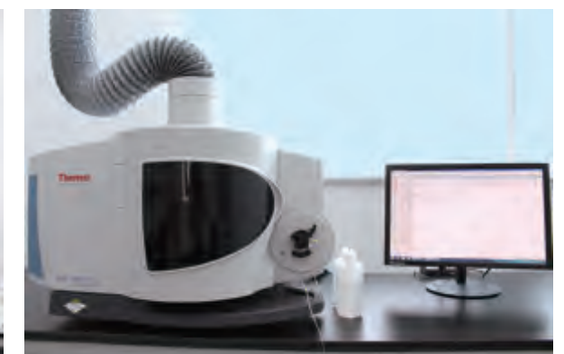
美国THERMO FISHER等离子体发射光谱仪 American Thermo Fisher plasma emission spectrometer
