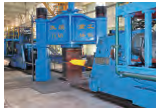
快速锻造车轴生产线 Production line for fast forging axles
